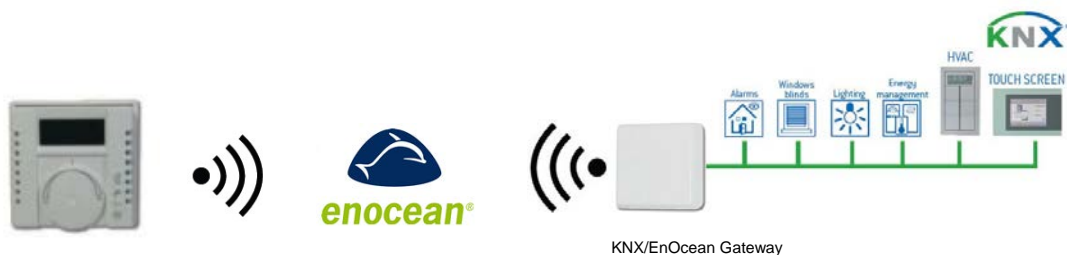
Figure 3.5 KNX/EnOcean Gateway and Rocker integration example
