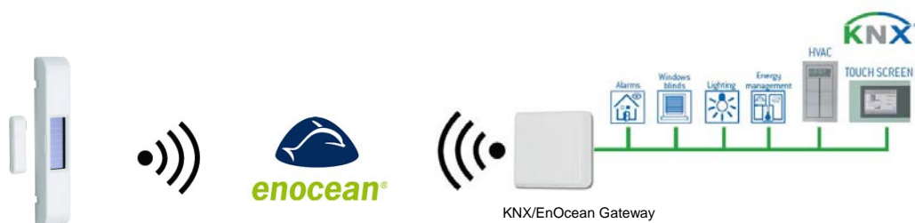
Figure 3.4 KNX/EnOcean Gateway and Window Contact integration example
