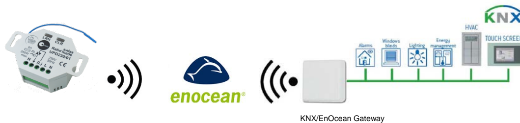
Figure 3.2 KNX/EnOcean Gateway and light actuator integration example
