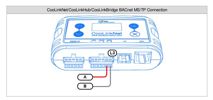
In CooLinkNet/CooLinkHub/CooLinkBridge devices only Line L3 can be used for BACnet MS/TP connection.
