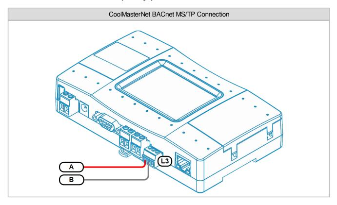
In CoolMasterNet Line L3 is recommended for BACnet MS/TP connection, although Lines L4, L5, L6 and L7 can also be used for that purpose. Picture above shows connection to Line L3.
