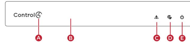
**A Data LED**—The Data LED shows solid red when the controller is streaming audio.
