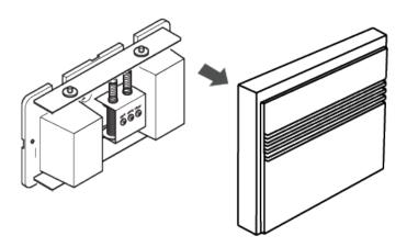
2. Wire the two wires from the chime adapter parallel to the wiring to the doorbell button where the VDB is installed.
