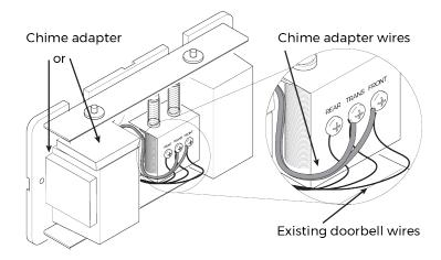
3. Remove the backing covering the adhesive on the chime adapter and adhere the chime adapter to the doorbell chime.
