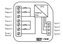
As indicated Power 2 is not tied to the neutral or input terminals, care must be taken if power is sourced from a different RCD to alleviate tripping.
