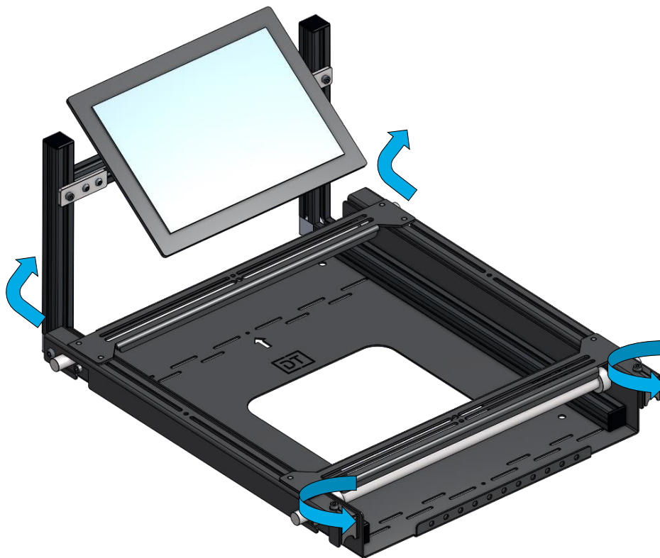
Fig.1. Removing the projector mount plate
