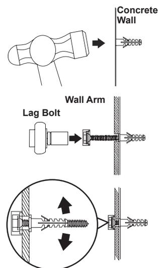
**CONCRETE must be 2500psi density minimum. Lighter density concrete may not hold concrete anchor.** Make sure that the supporting surface will safely support the combined load of the equipment and all attached hardware and components.
