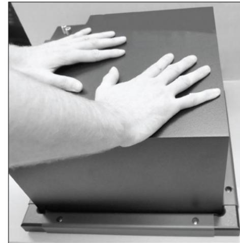
**F** Firmly press subwoofer down to seat it securely into the frame.
