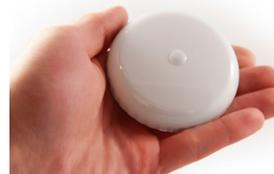
These sensor solutions combine the features of a motion sensor and ZigBee radio into a single small device. Packed with intelligent features, the wireless motion sensor expands Control4's network possibilities, reporting motion anywhere in the home, allowing the lighting system to respond accordingly. And all without any wires.
