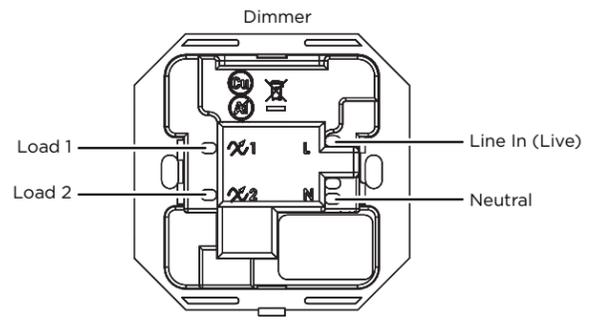
Figure 3: Single device location, without neutral connection
