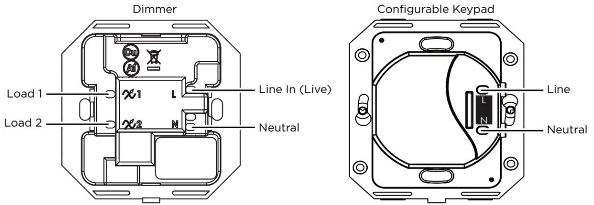
Figure 5: Multiple device locations using Configurable Keypad, without neutral connection at dimmer
