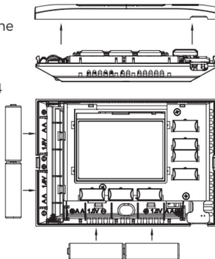
**✓ Important:** When batteries are replaced, all four batteries should be replaced with new alkaline AA batteries. Do not mix old and new batteries.
