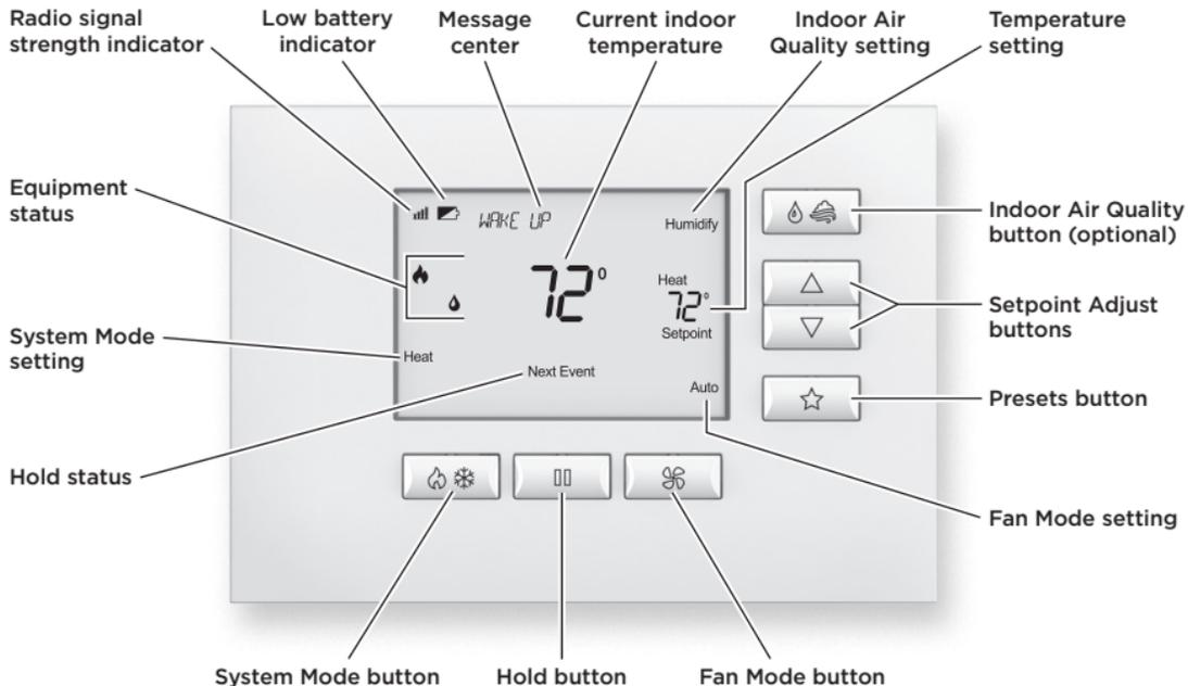
**Note:** Backlight is activated with the first button press and automatically turns off.
