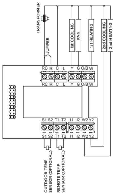
*Two transformers (remove jumper wire)*
