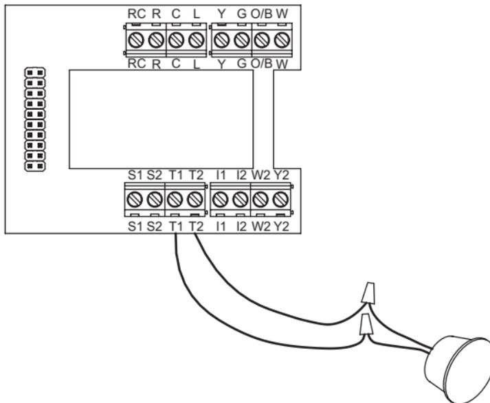
**The remote temperature sensor should be mounted:**
