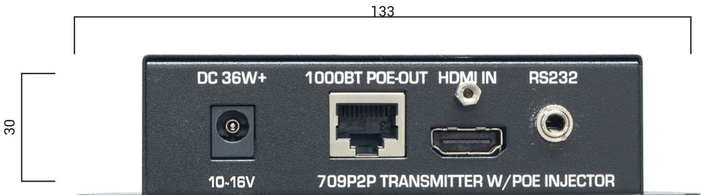
All measurements in millimeters (mm)
